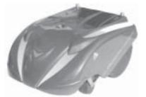
This robot will mow the lawn. Mowbot is equipped with bump sensors which are activated when it encounters an object; it then moves in the opposite direction.
