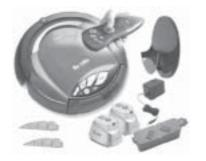
The image above is of a house-bound vacuum robot which can navigate a room avoiding obstacles while cleaning the carpet. The robot initially sweeps the room in a spiral pattern, and when an object is detected by the infrared sensors the guidance system plans a path to avoid collision. Once the job is finished, the robot will switch itself off.
